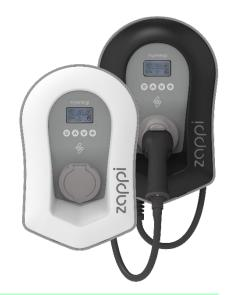
zappi has 3 charging modes which makes it great for all homeowners. Those with grid-tied microgeneration systems like wind or solar can use the eco setting to save on their energy bills. The charging current is automatically and continually adjusted in response to on-site generation and household power consumption. In FAST charge mode, zappi operates like an ordinary EV charging station.
